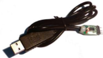
Connect the update cable to a free USB port of your computer. The FeedCarV2 is connected with the update cable and **only then the 5V operating voltage is applied**. The red LED on the FeedCarV2 is now blinking permanently. Then start the AVRrootloader tool on the computer, define the COM port under port and set the baud rate to 9600 Baud. With a mouse click on the „Connect“ button a connection to the FeedCarV2 will be established.
