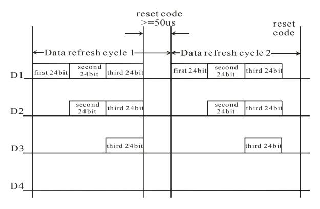
Note: The data of D1 is send by MCU, and D2, D3, D4 through pixel internal reshaping amplification to transmit.
